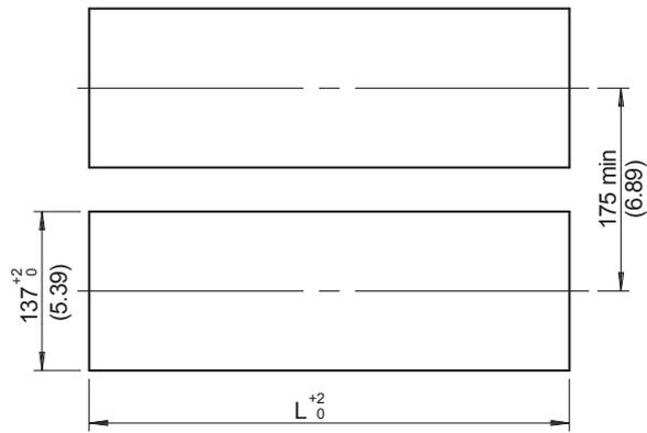
Side-by-side Mounting (vertically, max. 3 units)
