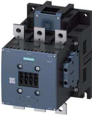
Power contactor, AC-3 265 A, 132 kW / 400 V AC (50-60 Hz) / DC operation 220-240 V UC Auxiliary contacts 2 NO + 2 NC 3-pole, Size S10 Busbar connections Drive: conventional screw terminal
