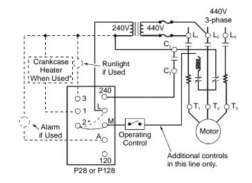
\*When crankcase heater is used, disconnect jumper 2 to M and reconnect 2 to L. Also, make sure that control circuit transformer has sufficient output for additional load.
