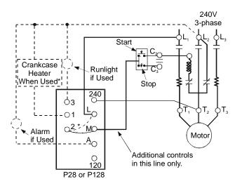
\*When crankcase heater is used, disconnect jumper from 2 to M and reconnect 2 to L.
