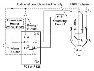
\*When crankcase heater is used, disconnect jumper from 2 to M and reconnect from 2 to L.
