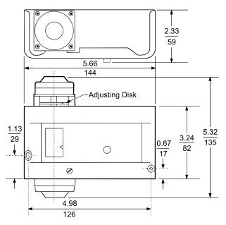
Figure 2: P28 or P128 Dimensions (in./mm)
