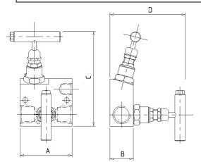
The 'G12AF' Type 2 valve manifold is designed for remote mounting to static pressure transmitters. The angled heads allow for panel mounting. The separate vent valve gives full control of venting of the instrument, plus the ability to calibrate in-situ. Each needle valve head is designed for safe and reliable isolation, giving bubble tight shut off, with non-rotating & anti-galling tip and dynamic self-adjusting spindle seal to give long service life in a variety of service conditions.
