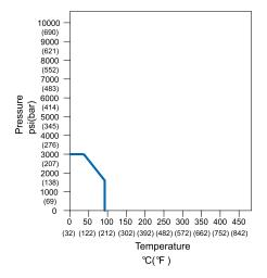
Graphs are based on 316 SS valves with PTFE stem packings.
