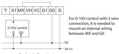
mount an internal wiring between MX and G0
